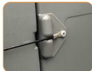
2-strain relief door springs
